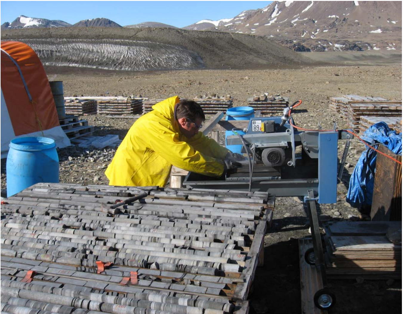
Cutting previously unassayed mineralised drill core on site at Citronen
